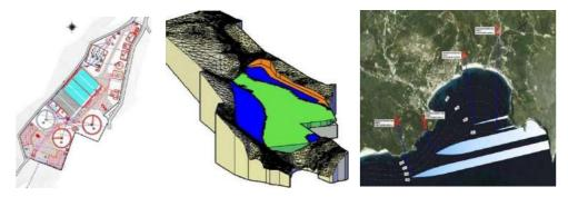
Left: Plan view of the WWTP, Middle: 3D terrain model, Right: Modelled effluent plume of sea outfall options
