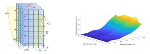
Figure 1. 16 story RC prototype frame building (left figure), wind directionality and wind intensity effects on the peak structural damage index (right figure)
